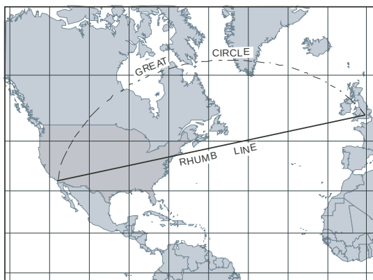
FIGURE 6.20. On the Mercator projection a great circle that is the shortest distance between two points on a sphere looks farther than the rhumb line. These distances can be compared on a globe.
